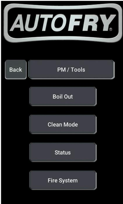
50. Clean Mode will allow for debris removal from the oil pot. The oil temperature must be above 250°F to access this feature.
