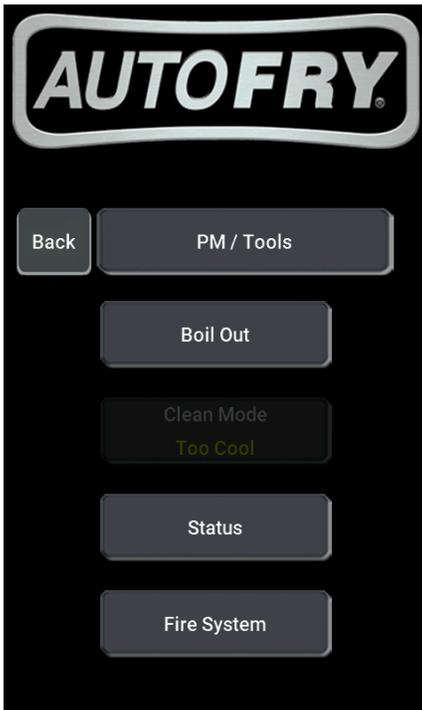
46. The Boil Out cycle will boil water for 15 minutes and then automatically shut off. Adding a cleaning agent such as Boil Out Pucks will improve the effectiveness.
