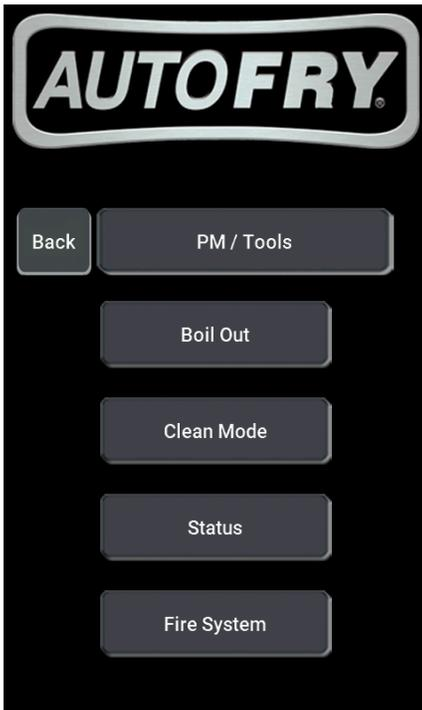
67. Fire System will show the date the fire system was last inspected and the next required inspection date.
