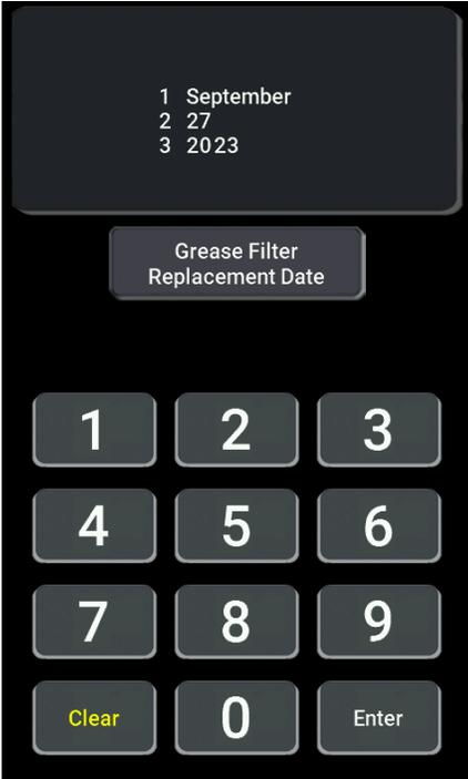
64. Press the Replaced date underneath Grease to edit the date the Grease Baffle was last replaced. Enter replaced date and press Enter to save.
